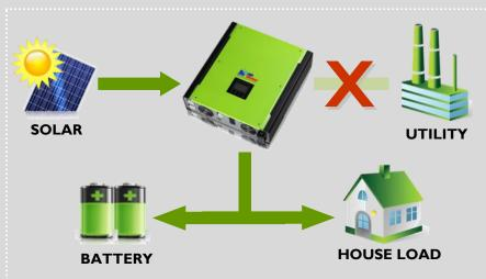
In this operation mode, grid feedback to utility is disabled. Users can only program unit to:
